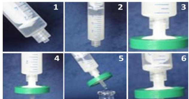
Fig-14: Luer lock membrane filter attached to a syringe
