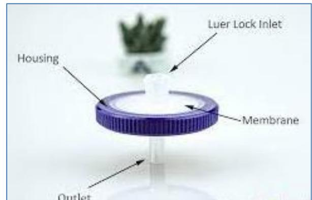
Fig-4.16: Luer lock syringe filter
