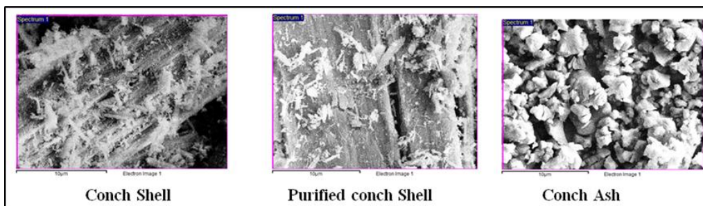
Fig 3: Surface Microphotograph (SEM) of all samples of Conch
