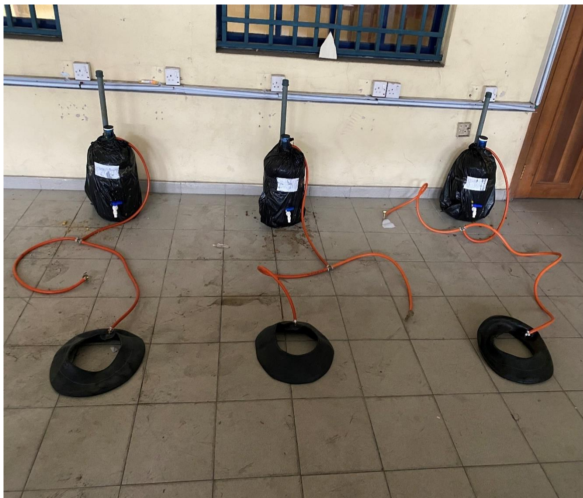
Figure 1: Experimental biodigester setup
