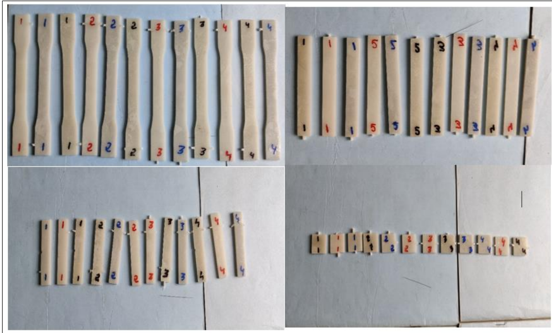
Fig. 4: Specimens for Mechanical Testing according to ASTM Standards
