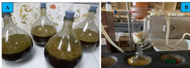
Figure 3: (a) Maceration method; (b) Soxhlet Extraction Apparatus
