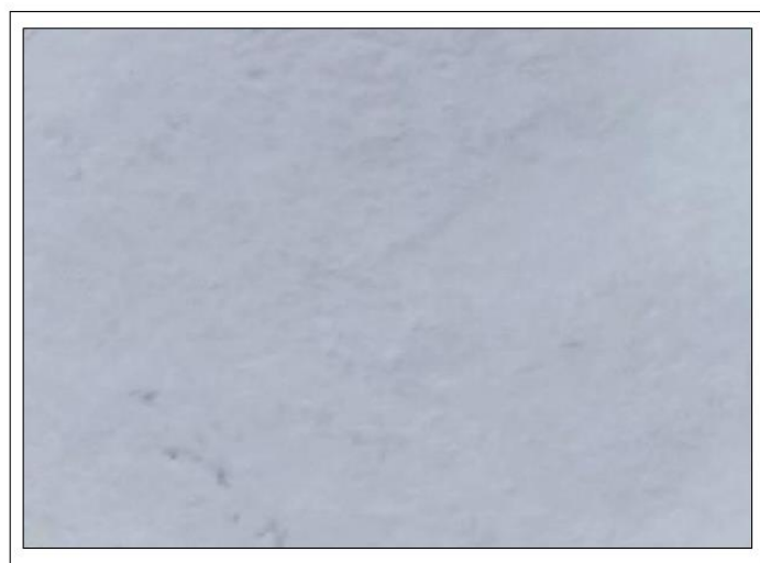
Fig 2: Handmade paper sheet produced from rice straw (Sample 3)
