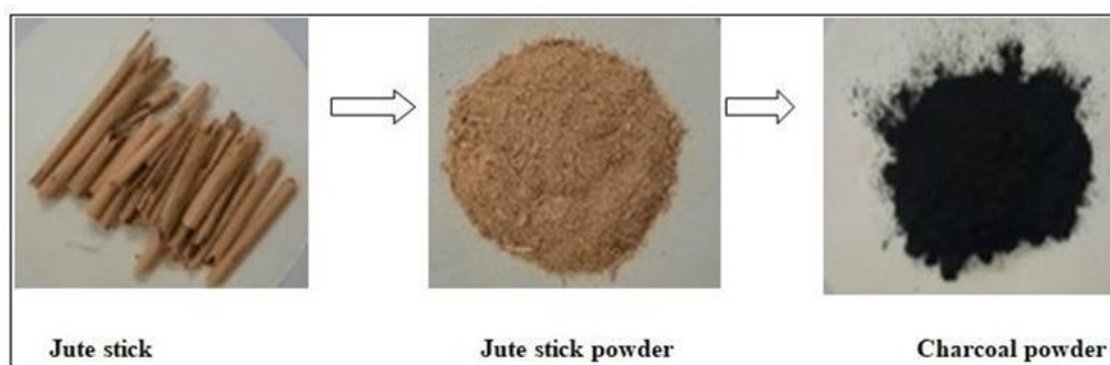
Fig 1: Preparation of activated carbon from jute sticks charcoal
