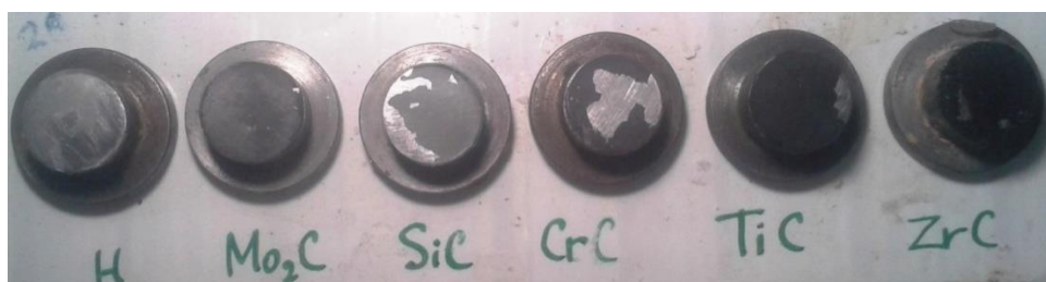
Fig 3: Films of epoxy-carbide adhesives in tearing-tested cylinders
