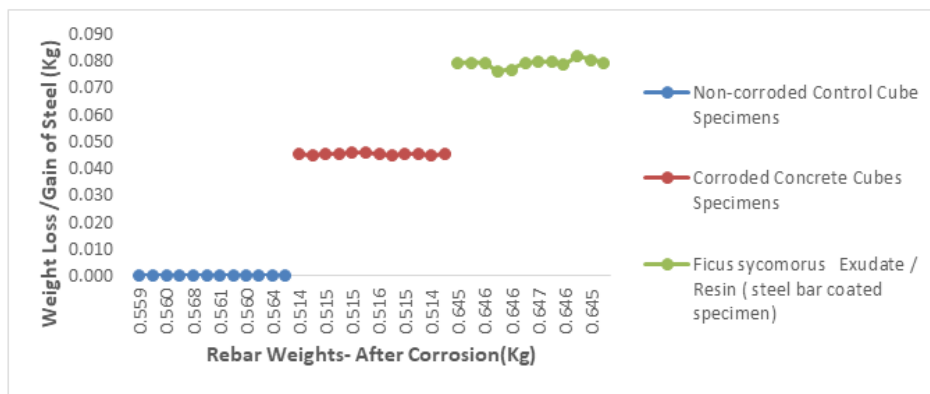
Figure 6: Rebar Weights- After Corrosion versus Weight Loss /Gain of Steel
