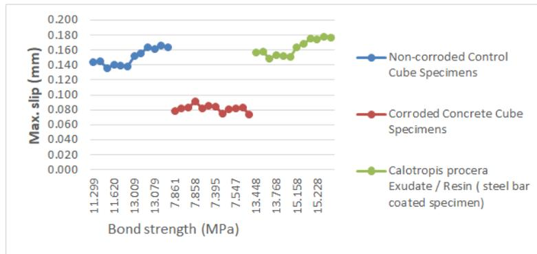
Figure 2: Bond Strengths versus Maximum Slip
