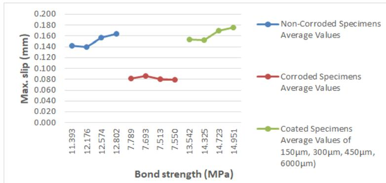
Figure 2a: Average Bond Strengths versus Maximum Slip
