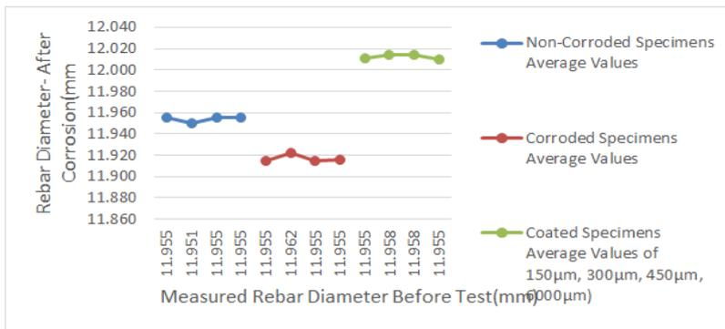
Fig 3a: Average Measured (Rebar Diameter before Test vs Rebar Diameter- after Corrosion)
