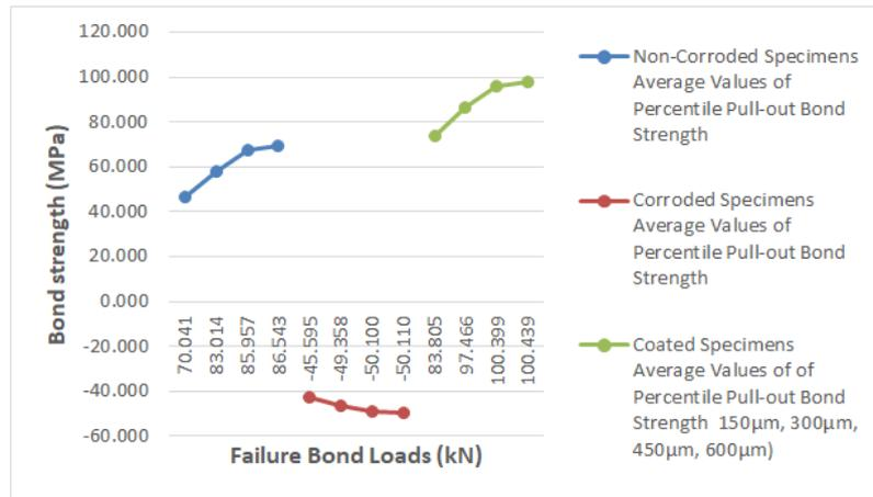
Figure 1b: Average Percentile Failure Bond loads versus Bond Strengths
