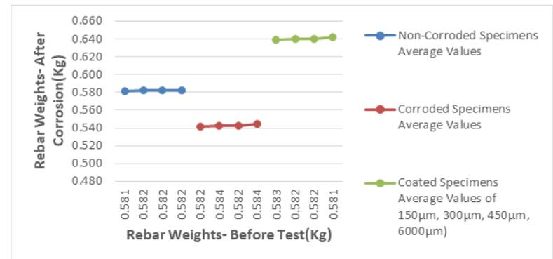
Figure 5a: Average Rebar Weights- before Test versus Rebar Weights- after Corrosion
