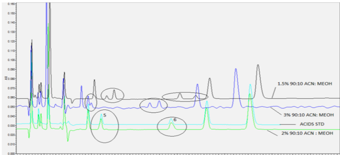
Fig-5: (D) Impact of mobile phase composition on the separation of organic acid peaks
