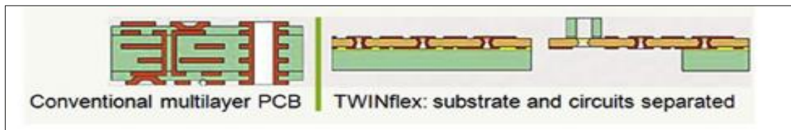
Figure 4: Conventional printed circuits board and the TWINflex concept [23]
